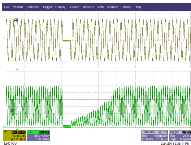
Figure 46 – 115 VAC / 50 Hz, 2 Cycle-Skip. Load: 35 V LED String. Ch1: V_{IN} , 50 V / div. Ch3: I_{IN} , 50 mA / div., 100 ms / div.
