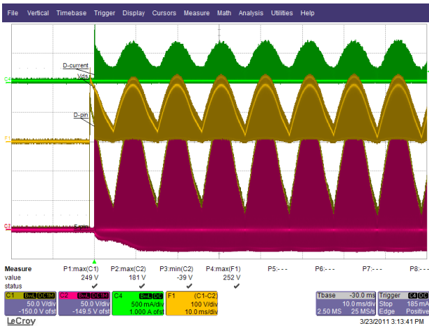
Figure 31 – 135 VAC / 63 Hz, 35 V LED String. Ch1: V_{DRAIN} , 50 V / div. Ch2: V_{SOURCE} , 50 V / div. Ch4: I_{DRAIN} , 0.5 A / div. F1: V_{D-S} , 100 V / div., 10 ms / div.
