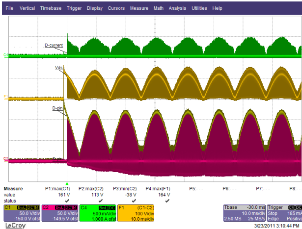
Figure 29 – 85 VAC / 47 Hz, 35 V LED String. Ch1: V_{DRAIN} , 50 V / div. Ch2: V_{SOURCE} , 50 V / div. Ch4: I_{DRAIN} , 0.5 A / div. F1: V_{D-S} , 100 V / div., 10 ms / div.
