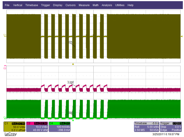
Figure 42 – 115 VAC / 50 Hz, 1 s On - 1 s Off. Load: 35 V LED String. Ch1: V_{IN} , 50 V / div. Ch2: V_{OUT} , 10 V / div. Ch4: I_{OUT} , 100 mA / div., 5 s / div.
