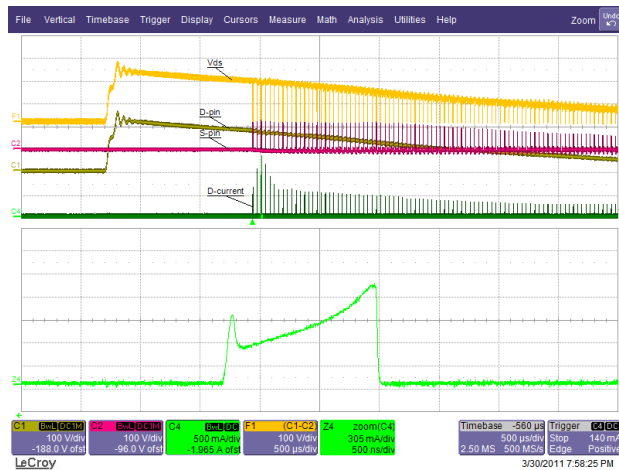
Figure 34 – 150 °C Start-up; 135 VAC / 63 Hz; 85° Phase Angle, 35 V LED String. Ch1: V_{DRAIN} , 100 V / div. Ch2: V_{SOURCE} , 100 V / div. Ch4: I_{DRAIN} , 0.5 A / div. F1: V_{D-S} , 100 V / div., 500 μs / div. Z4: I_{DRAIN} , 305 mA / div.; 500 ns / div.
