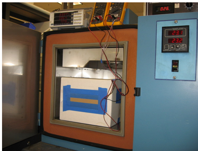
Figure 18 – Thermal Chamber Set-up Showing Box Used to Prevent Airflow Over UUT.
