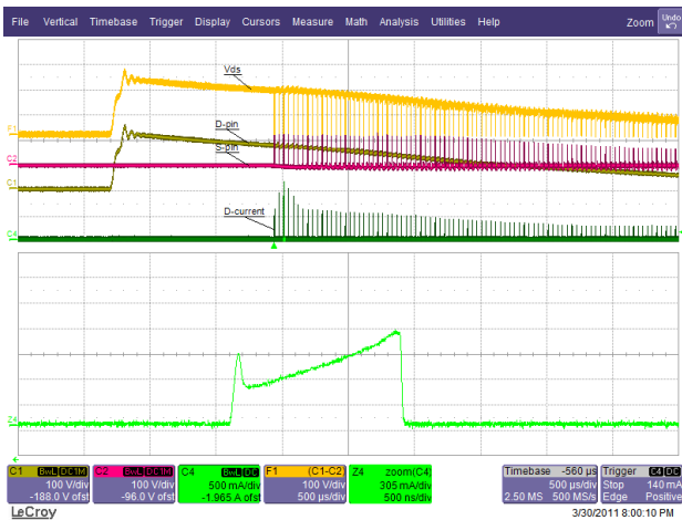
Figure 33 – 125 °C Start-up; 135 VAC / 63 Hz; 85° Phase Angle, 35 V LED String. Ch1: V_{DRAIN} , 100 V / div. Ch2: V_{SOURCE} , 100 V / div. Ch4: I_{DRAIN} , 0.5 A / div. F1: V_{D-S} , 100 V / div., 500 μs / div. Z4: I_{DRAIN} , 305 mA / div.; 500 ns / div.
