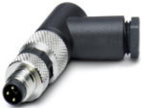
Connector, 3-position, Plug angled M8, A-coded, Screw connection, Knurl material: Nickel-plated brass, External cable diameter 3.5 mm ... 5 mm
