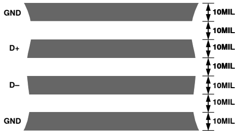
Figure 19. Arrangement of Signal Tracks
